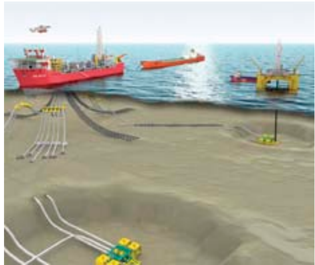
The Terra Nova FPSO is designed to hook up to the reservoir.
